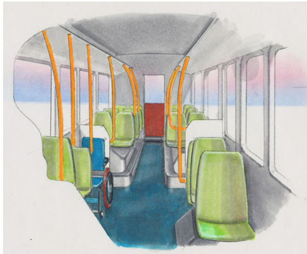
Fig. 13 The interior of an large-size electric full-flat bus with a low floor designed by Seijiro NODA
