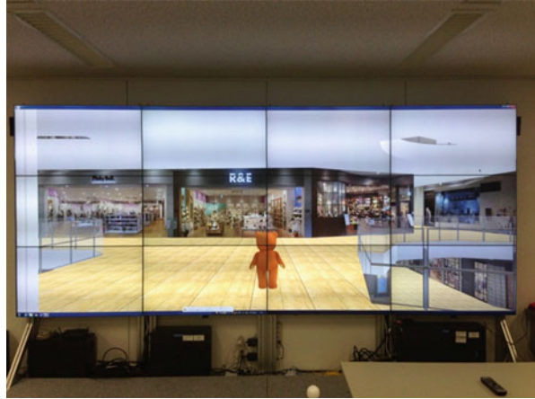
Fig. 11 Visualized virtual position of the subject as a teddy bear on the tiled wall display
