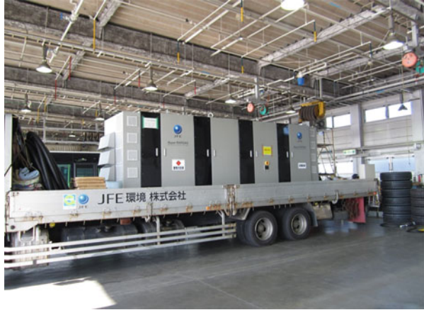
Fig. 9 The overly rapid electric supply machine tried this time (ELFB becomes full in about 30 min from SOC 50 %)
