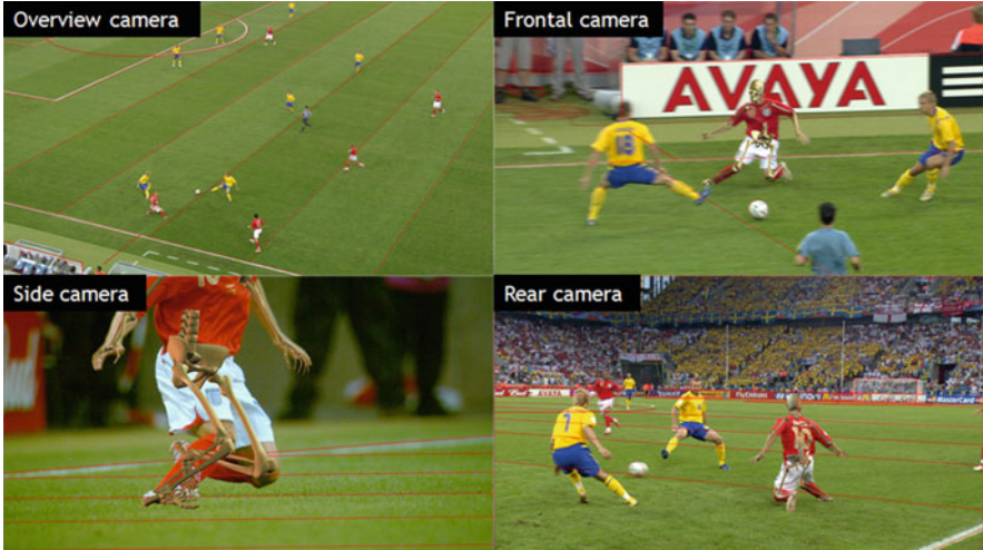
Fig. 10.4 A soccer injury situation recorded using HD cameras. Each panel shows the customized skeleton model and the football pitch model superimposed on and matched with the background video image from each camera. Overview camera and rear camera had an effective frame rate after being deinterlaced of 50 Hz, frontal camera 100 Hz, and side camera 300 Hz
