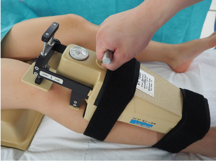
Fig. 11.1 The KT-1000 arthrometer has been widely used for diagnosis and preoperative and postoperative evaluation of ACL-deficient knees, because of its accuracy and reproducibility in the measurements of tibial anterior/posterior translation
