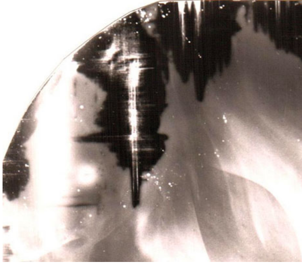
Fig. 9.14 Dark field image of part of a wafer which had undergone excessive temperature stress (during rapid thermal anneal as part of a haze test), where the dislocation arrays in the [100] direction are well visible via the etch pits of the dislocations (additionally visible: haze from metal contamination, which is not present in the dislocated areas due to gettering of the metal impurities by the dislocations). The wafer has been defect etched to show develop etch pits where the dislocation penetrate the surface, the light scattering from the etch pits shows up the intersection of the glide planes with the surface, where a high density of etch pits shows up as lines in the \langle 110 \rangle directions, also compare Fig. 9.7
