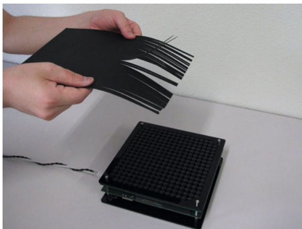
Fig. 8.6 Focused ultrasound flips up paper strips
