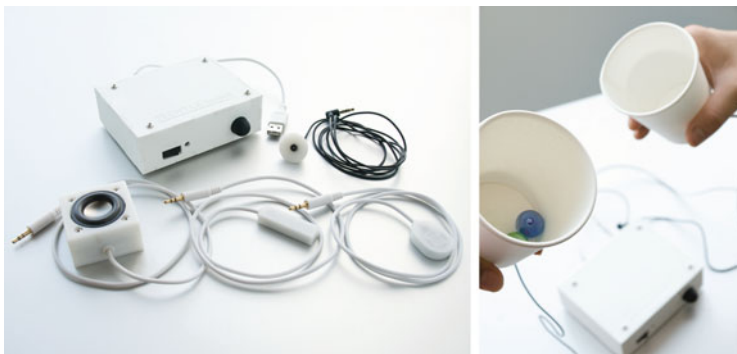
Fig. 12.2 The TECHTILE toolkit that can record and play back haptic experiences ( left ). An example of the transmission of the haptic content related to feelings a glass ball in a cup ( right )
