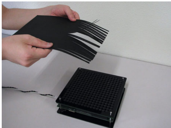
Fig. 8.6 Focused ultrasound flips up paper strips
