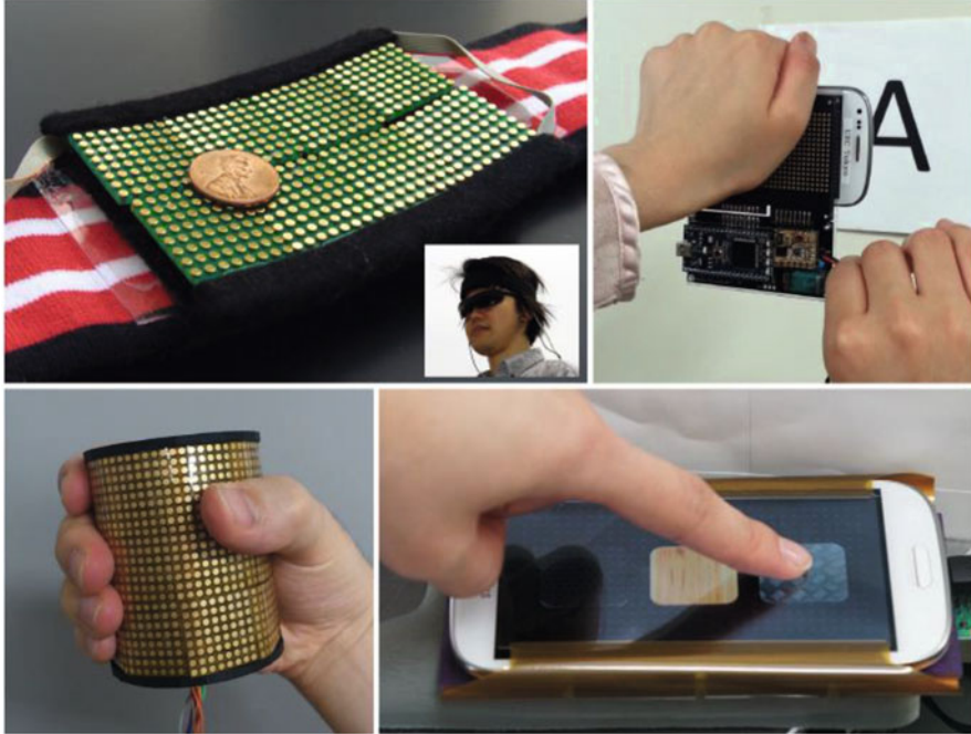
Fig. 5.1 Applications of the electro-tactile display. ( Top left ) Forehead stimulation for a tactile-vision substitution system (TVSS) [1]. ( Top right ) TVSS of palm type [4]. ( Bottom left ) Cylindrical type for virtual-reality application [5]. ( Bottom right ) Touch-panel type using transparent electrodes [6]
