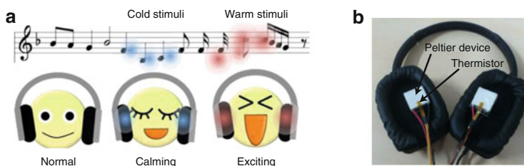
Fig. 11.8 (a) Concept of ThermOn (b) Headphone-type device using a Peltier device [29]
