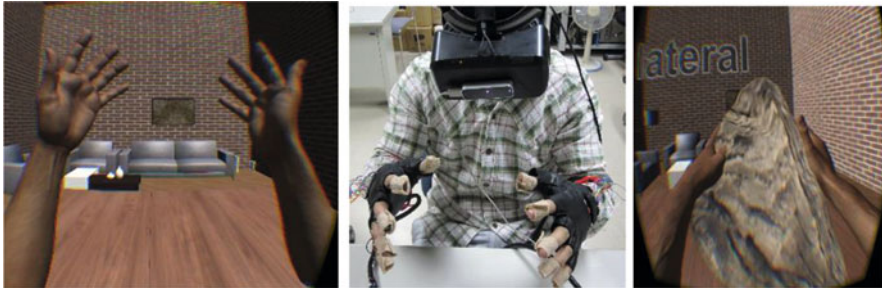
Fig. 4.21 System for presenting pseudo-tactile sensations in VR Space
