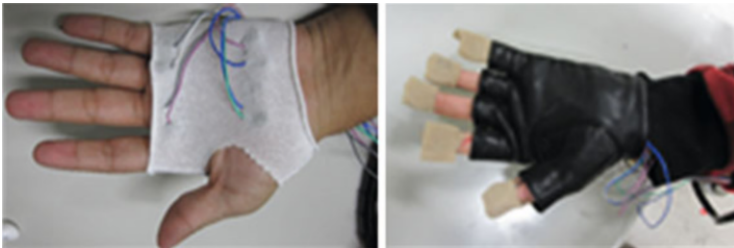
Fig. 4.19 Tactile glove and its nine tactile actuators inside
