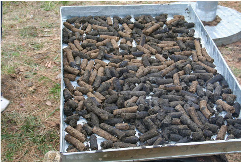
Fig. 12.23 A rod-shaped piece of fuel is produced by inserting burned and carbonized yak dung into the device (This photograph was provided by Mr. Dutta of the World Wildlife Fund (WWF))
