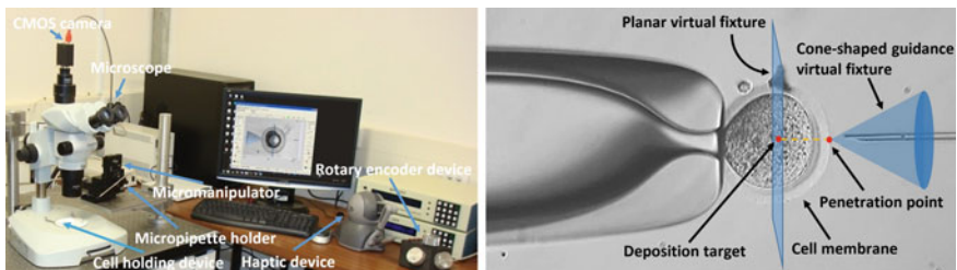
Fig. 1 Physical haptic micro-robotic cell injection system ( left ); visualisation of haptic virtual fixtures ( right )
