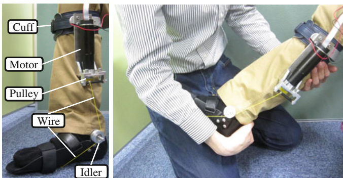
Fig. 1 Exoskeletal ankle simulator and training scene
