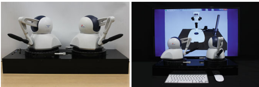
Fig. 2 Reconfigurable multipurpose haptic interface [13] ( left ); haptic VR training environment for cell injection ( right )
