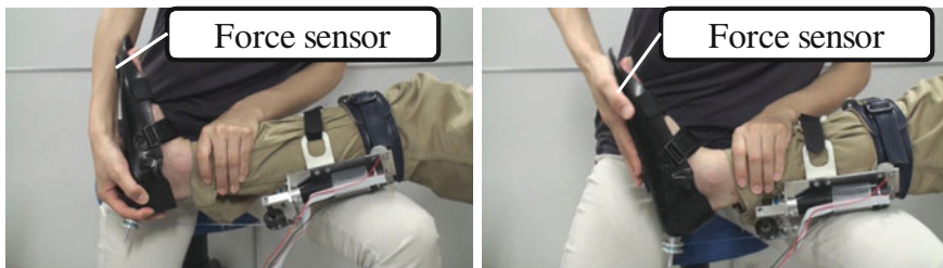
Fig. 2 Measurement setup; left spasticity test and right clonus test
