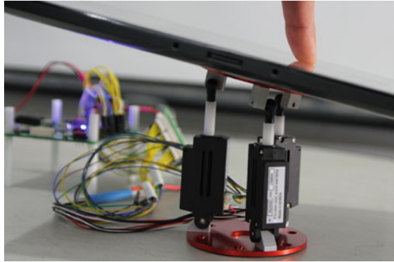
Fig. 2 Proposed robotic surface based on a simple RPS parallel platform. The surface orientation based on the touched 3D geometry would provide immersive visual and haptic experiences
