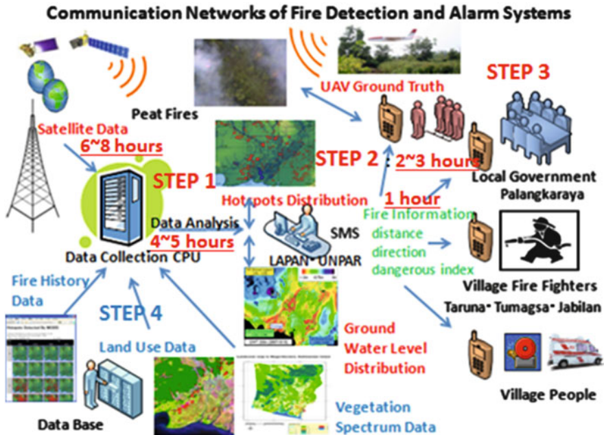
Fig. 26.1 Fire communication networks
