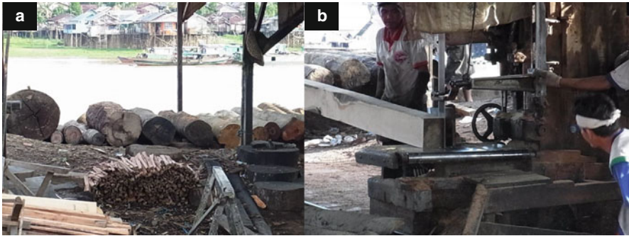
Fig. 35.5 Sawing a log for local use in a lumber mill in Palangka Raya, Central Kalimantan, Indonesia. (a) Logs transported in the river. (b) Belt-saw at work
