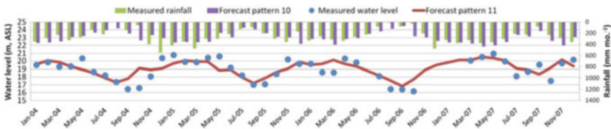
Fig. 16.11 Results of rainfall forecasting and of water level forecast using forecast rainfall (1 month lead time)
