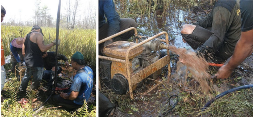
Fig. 27.6 A large amount of water in the aquifer below peat layer
