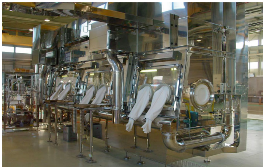
Fig. 13.1 Investigational New Drug (IND) vial-ampoule manufacturing machine Clinical Scale vialampoule aseptic processing isolator system
