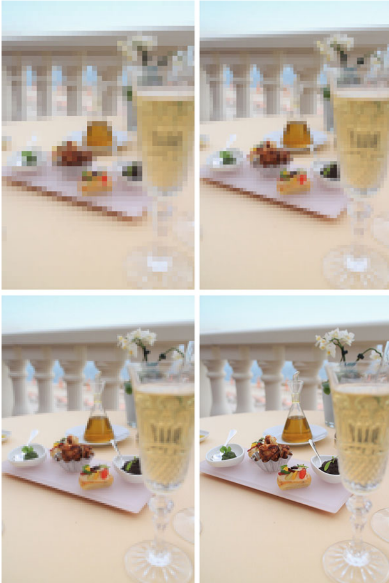
Fig. 1.2 Effect of pixel size on image quality. Number of pixels are 2.2 k, 5 k, 20 k, and 18 M, respectively, left to right
