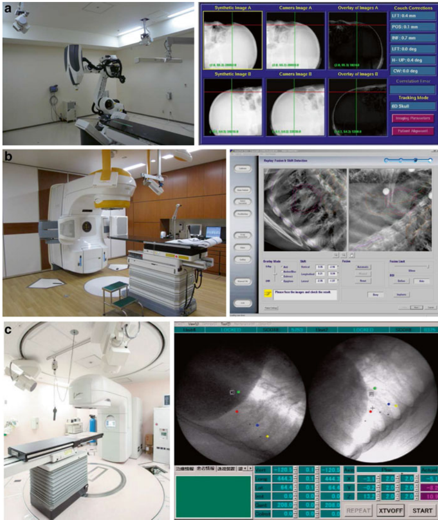
Fig. 5.9 2D kV stereoscopic imaging systems. (a) The CyberKnife system. (b) The Novalis Linac system with the ExacTrac imaging system. (c) Real-time tumor-tracking radiotherapy system
