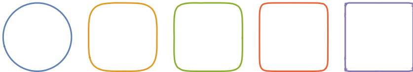
Fig. 2 The Wulff shapes W_{(p)} for the energy density \gamma_{(p)} in (10). W_{(1)} is a circle. When p approaches infinity, W_{(p)} converges to a cube
