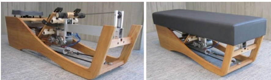
Fig. 25.4 A new type of indoor rowing ergometer, the e-Rowing ergometer ( left ). After training, the e-Rowing ergometer can be converted to a bench with cover ( right )
