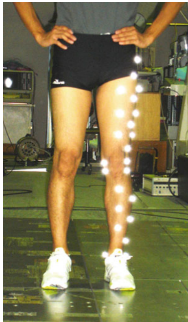
Fig. 29.1 Arrangement of markers for the point cluster technique. Twenty-five reflective markers were secured to the left lower extremity of each subject ( This is the Author's Accepted Manuscript of an article published as "Change in tibial rotation of barefoot versus shod running." as published in Footwear Science Vol.1, No. 1 March 2009, 19–23 copyright Tylor & Francis, available online at http://www.tandfonline.com/ , doi:10.1080/19424280902950456 )
