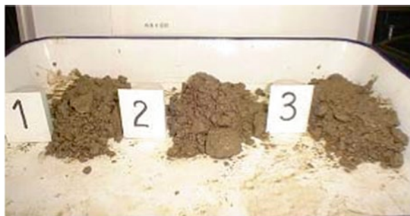
Cement-stabilized soil after 2 nd cycle
