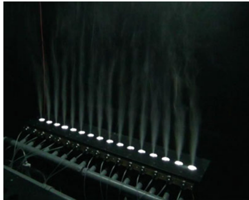
Fig. 16.6 Nanofiber spinning with 16 nozzles by blow electrospinning (BES)
