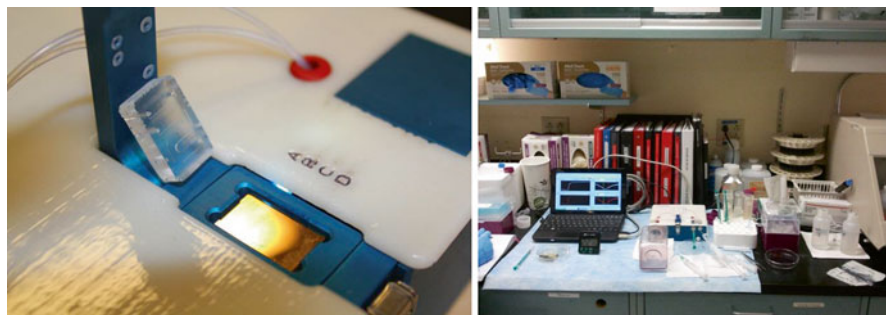
Fig. 15.13 Left : The four-channel SPR instrument was designed based on a 20 \times 12 mm dove prism. A fluidic cell delivers the sample to three channels for a triplicate measurement and a fourth channel serves as the reference. Right : The system takes little space in a laboratory. The total space needed to run experiments is less than 1 \text{ m}^2 . No external power is required to run the instrument, making it portable. Reproduced from Zhao et al. (2015) with permission from Elsevier
