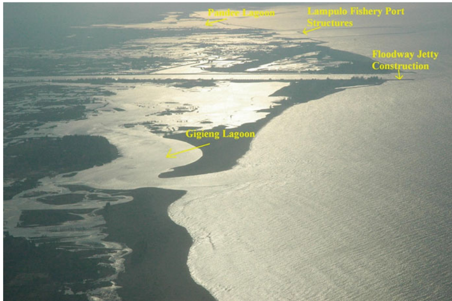
Fig. 13.3 The Pandee Lagoon ( upper part ) and the Gigieng Lagoon ( middle part of the picture ). The picture shows the coastal lagoons condition in February 2013. Floodway jetty construction and the Lampulo fishery port structures are assumed to block the longshore sediment transport along the coastal area
