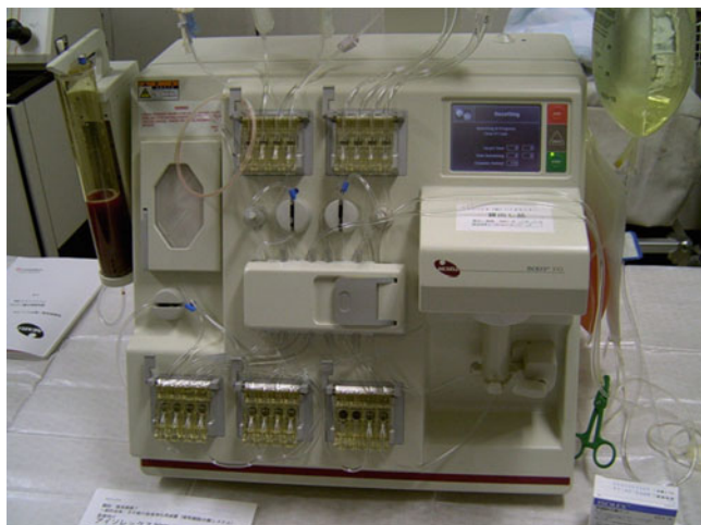
Fig. 29.2 Isolex300i magnetic cell selection system separates CD34 + cells from the fraction of mononuclear bone marrow cells for about 3 h
