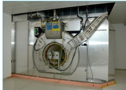
First generation high field MRI-guided radiation therapy system is now under test
