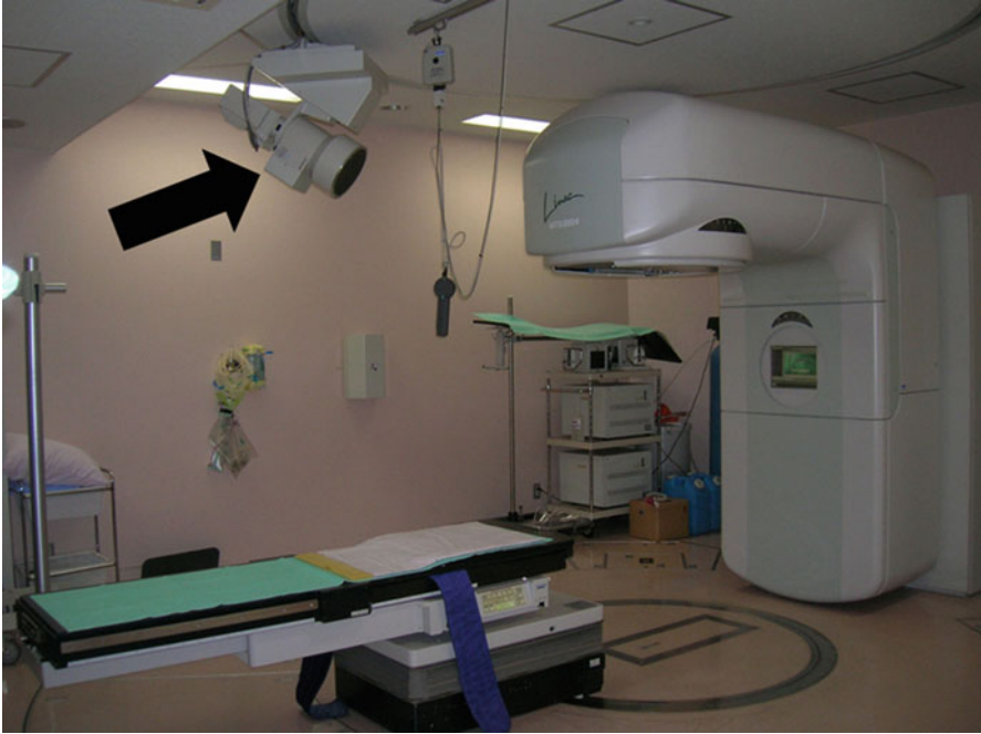
Fig. 17.1 RTRT system in Hokkaido University. Black arrow shows the image intensifier (I.I.)
