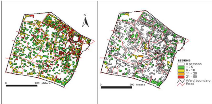
Fig. 6.6 Buildings collapse probability ( left ) and potential casualty ( right ) at MMI IX level of shaking
