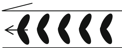
Fig. 9.24 The smectic layer structure formed by banana molecules. The banana molecules are packed into a layer with the same directionality, showing the spontaneous polarization along the bent direction
