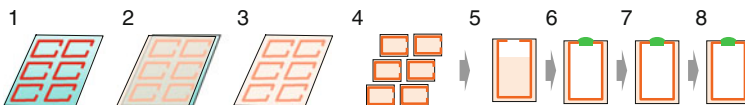
Fig. 7.14 Process of vacuum injection method. (1) Sealant dispensing. (2) Sealing. (3) Thermal curing. (4) Cutting. (5) LC filling. (6) End filling. (7) UV curing. (8) Thermal curing
