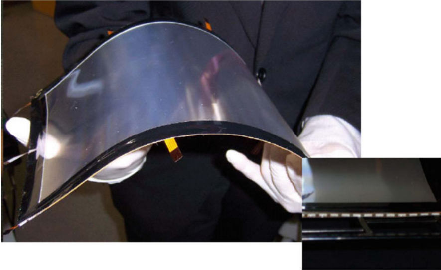
Fig. 8.12 Flexible light-guide plate backlight using small light-emitting diodes
