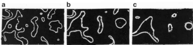
Fig. 3.2 Reverse-tilt disclinations in a TN cell (©IEEE Tr.ED)
