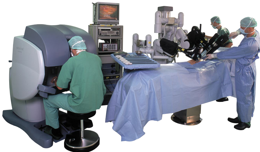
Fig. 2.1 The da Vinci ® Standard Surgical System
