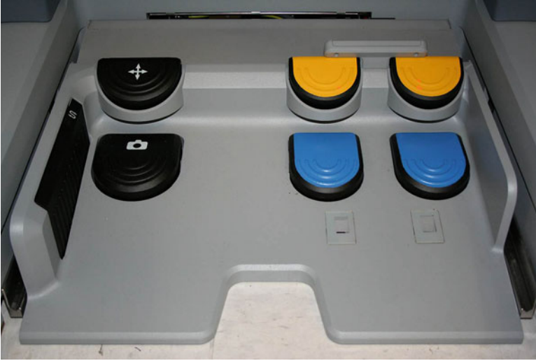
Fig. 2.7 The da Vinci® footswitch panel
