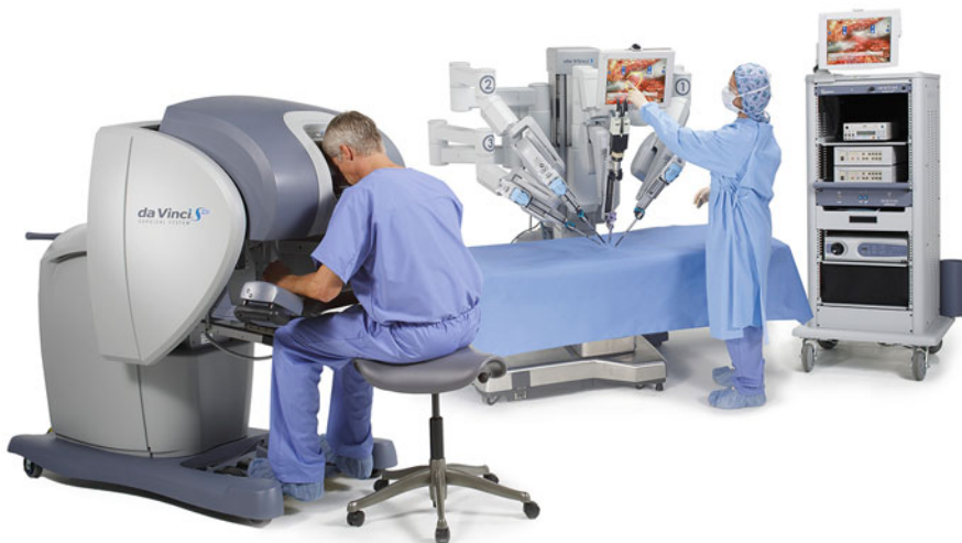
Fig. 2.2 The da Vinci ® S Surgical System
