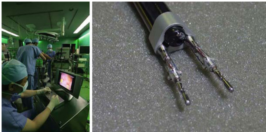
Fig. 1.1 Endoscopic robot system for NOTES
