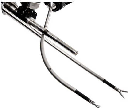
Fig. 2.11 The da Vinci ® single-site instruments
