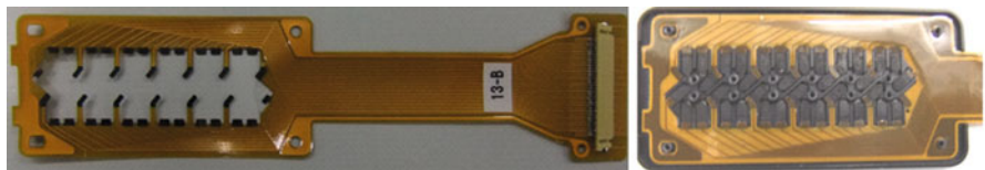
Fig. 27.6 FPC for wiring and wired actuators
