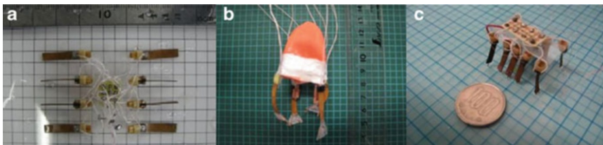
Fig. 29.4 Prototype microrobots. (a) Stick insect-inspired [2], (b) Jellyfish-inspired [1], (c) Inchworm-inspired [25, 31]
