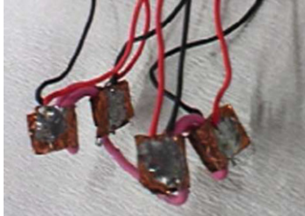
Fig. 28.7 Skeletal wire and the copper electrode contacts [17]
