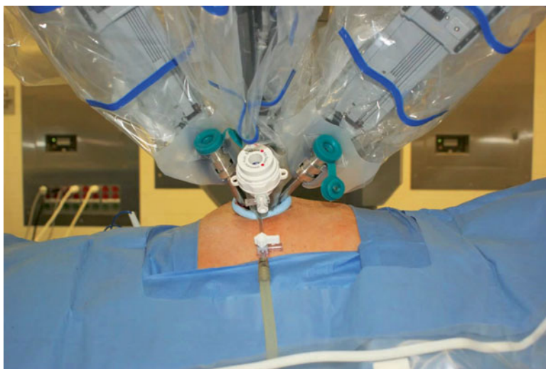
Fig. 2.7 Single Site daVinci (Intuitive). Single incision robotic surgery is already in clinical use
