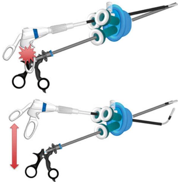
Fig. 7.13 Articulating forceps. Articulating forceps can be used to prevent handle clashing at hand when instruments are used in parallel
