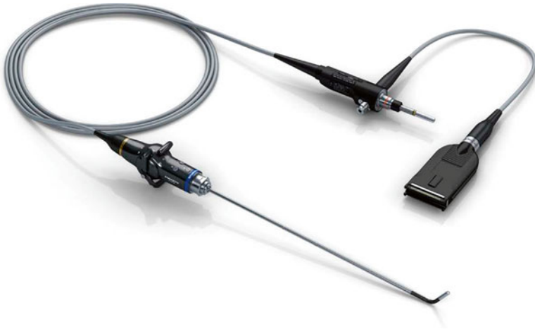
Fig. 7.5 LTF-S19-5 deflectable videoscope (Olympus). The tip of the scope can be moved 200° in four directions and the CCD/ light-guide cables are arranged in one line
