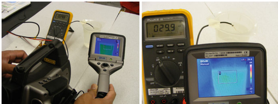
Fig. 10.2 Camera calibration was verified by taking measurements in warm- and cold-water baths by using the infrared camera and comparing the readings to those from a thermocouple at temperatures across the experimental range
