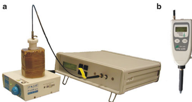
Fig. 8.5 Optical biosensors employing purified haloalkane dehalogenase: (a) instrumentation of the first biosensor prototype (25 × 7 × 25 cm, Bidmanova et al. 2010a) and (b) the fine-tuned and miniaturized latest version of the biosensor EnviroPen (6 × 3 × 19 cm, www.enantis.com )
