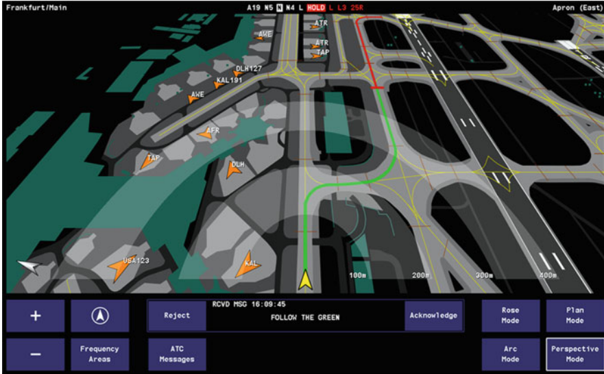
Fig. 2 HMI of the taxi guidance application (CDS)
