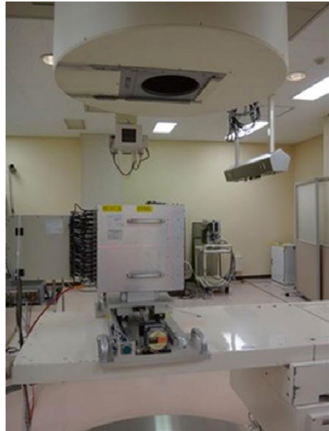
Fig. 8.2 MLIC set on the couch to measure the depth-dose distribution of vertical beam
