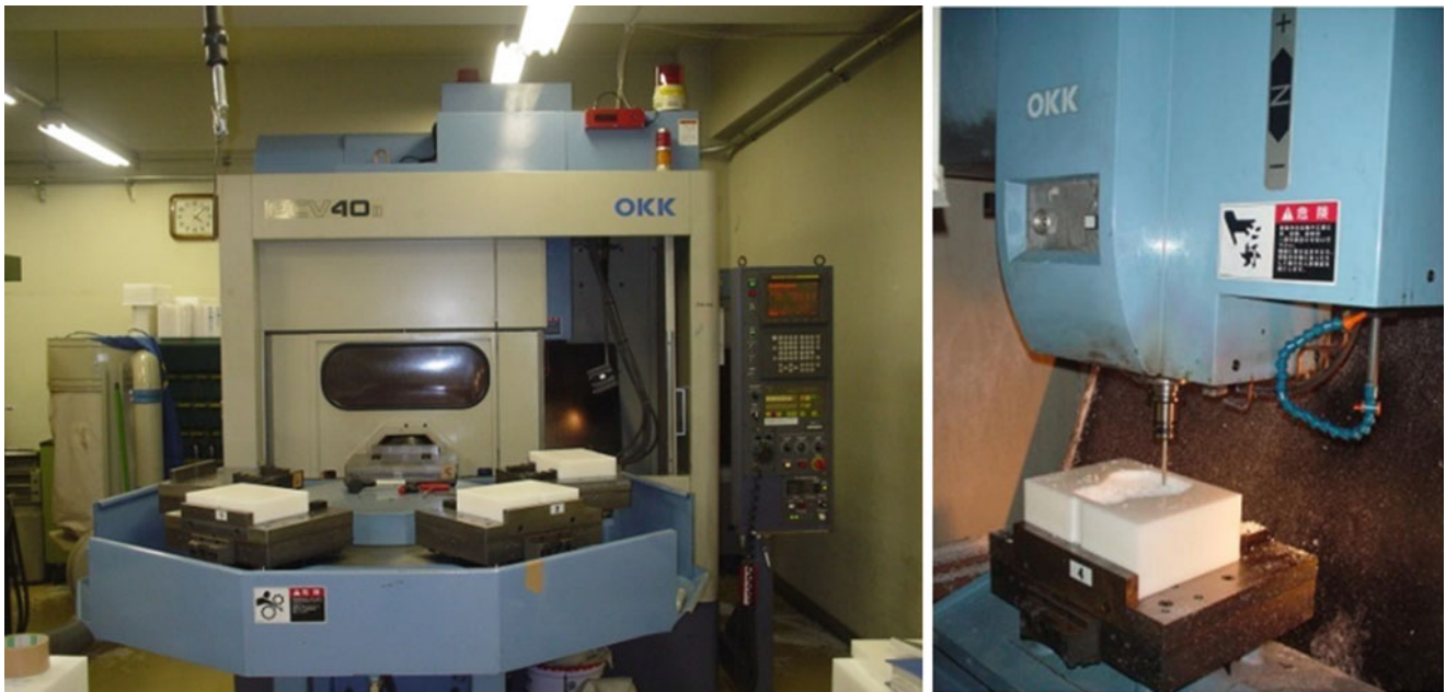
Fig. 7.5 Manufacture of patient compensators by machining center
