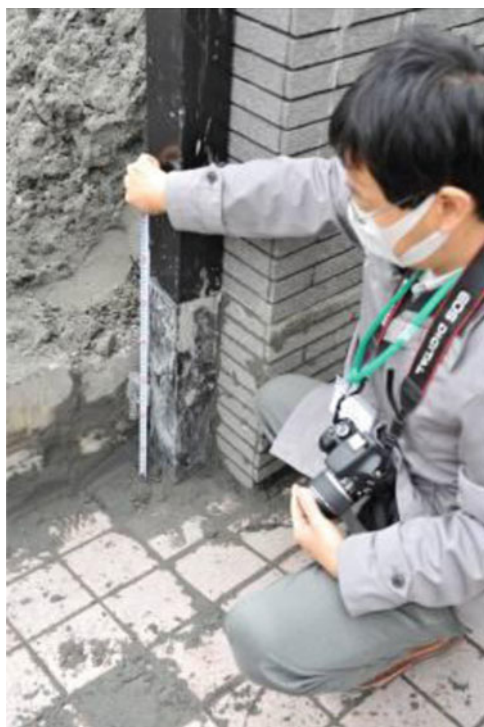
Fig. 10.5 55 cm accumulation of sand
