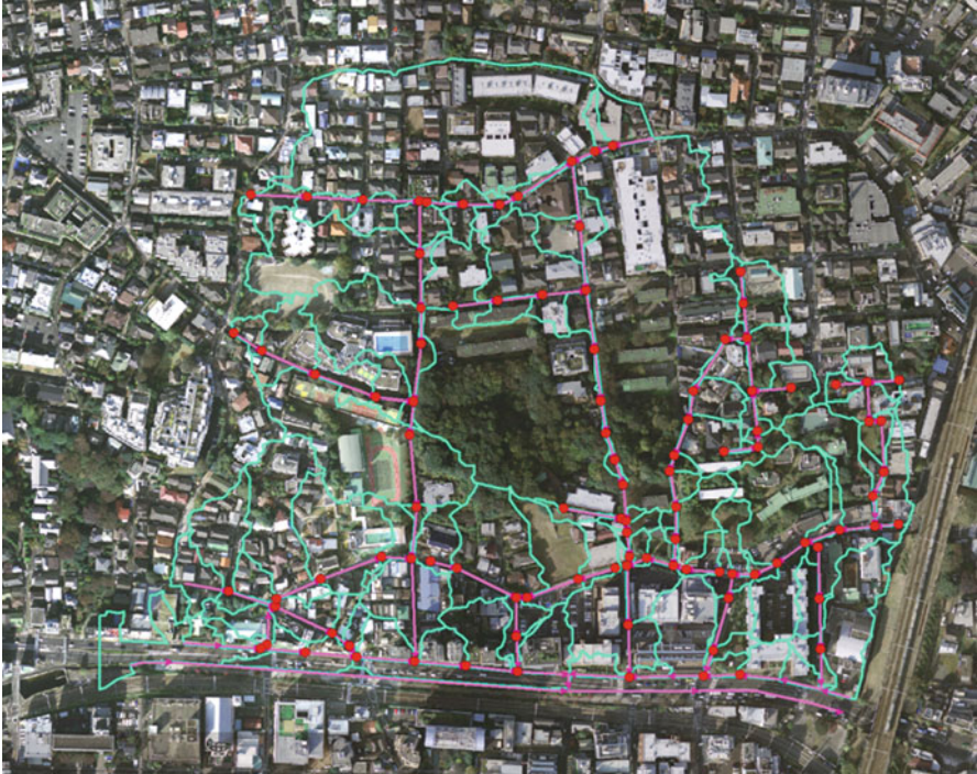
Fig. 3.23 Sewer catchment area adjacent to Otomeyama Park. Green line : sewer catchment area, Red Point : location of manhole
