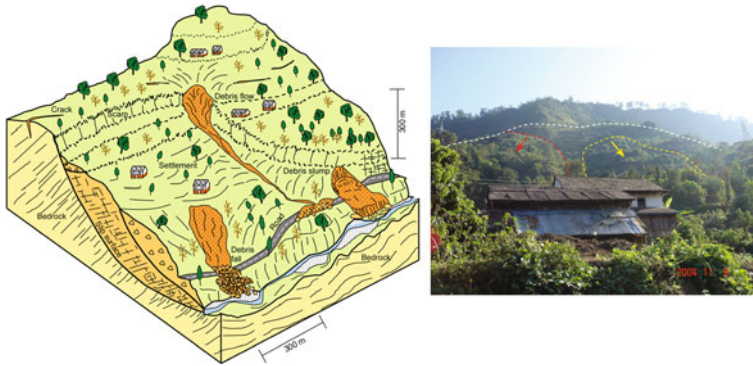
Fig. 6.5 Schematic diagram along with a photograph of a large-scale landslide and its characteristics features in the Lesser Himalayan Zone of Nepal. Red and yellow dotted lines (right photo) indicate two large-scale landslide masses moving in two different directions, also indicated by red and yellow arrows (right photo). Similarly, the white line (right photo) indicates the detachment zone or scarp
