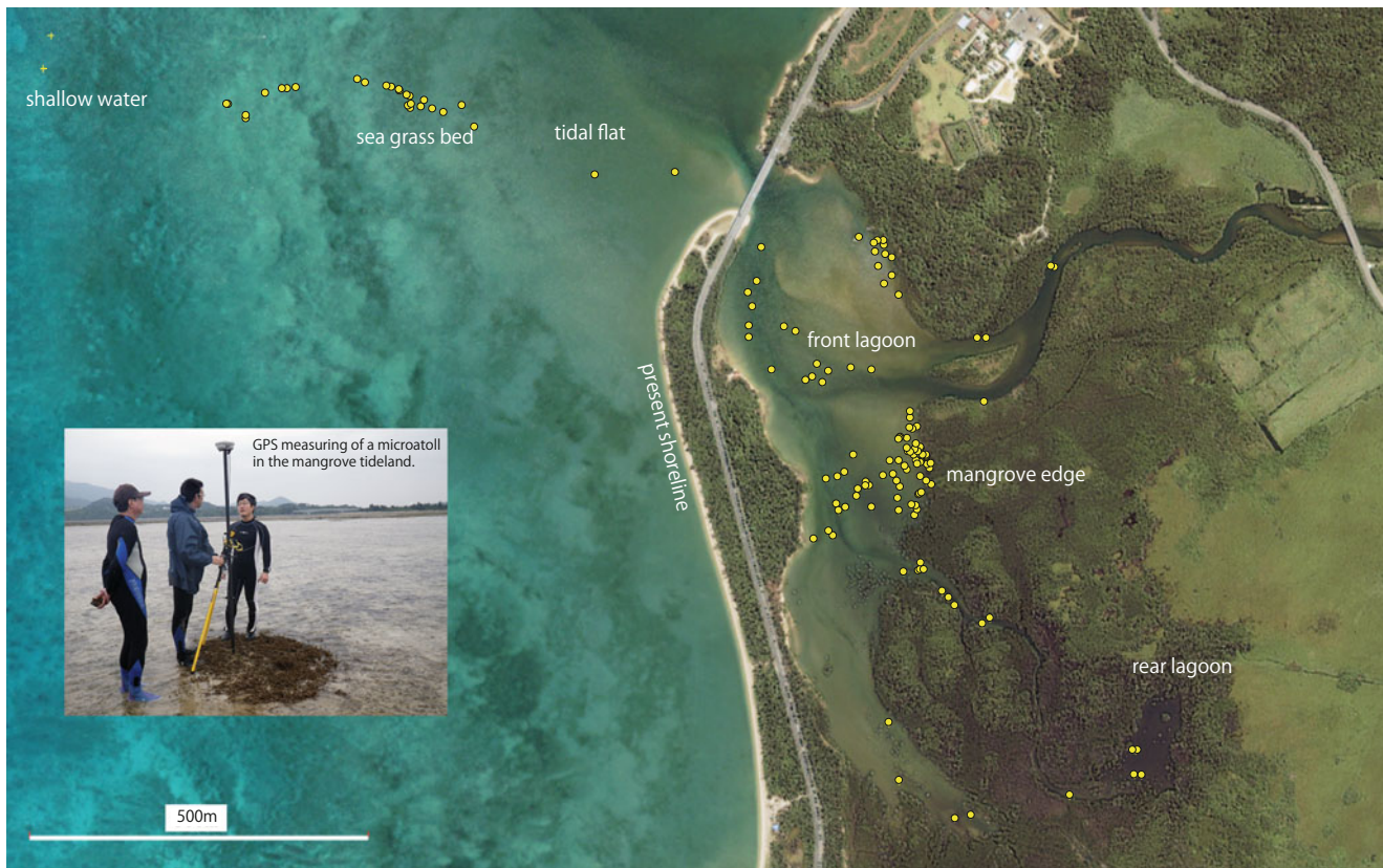
Fig. 4.2 We measured emergent Porites and Favia microatolls (yellow dots) in the mangrove tideland and along a transect in the tidal flat of the Nagura region by the RTK-GPS method. Several colonies of dead Porites (yellow crosses) were found lying at a depth of about 2 m
