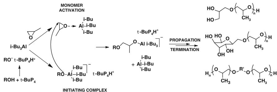
**Scheme 12** Combination of phosphazene base and *i*-Bu<sub>3</sub>Al for the synthesis of polyhydroxy telechelic PPO
