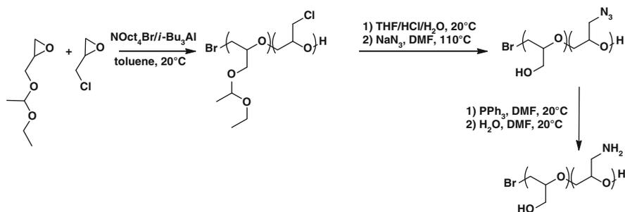
**Scheme 14** Synthesis of poly(glycidol-co-glycidyl amine) from protected glycidol and epichlorohydrin units
