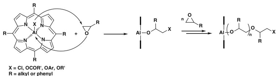
**Scheme 5** Polymerization mechanism of epoxides initiated by an aluminum porphyrin
