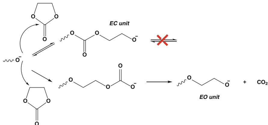
**Scheme 64** Mechanism of the AROP of ethylene carbonate
