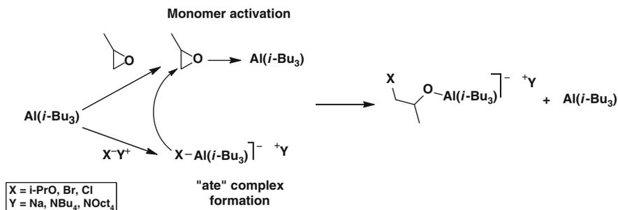
**Scheme 7** Nucleophilic attack of sodium alkoxide or ammonium salts/triisobutylaluminum on activated propylene oxide
