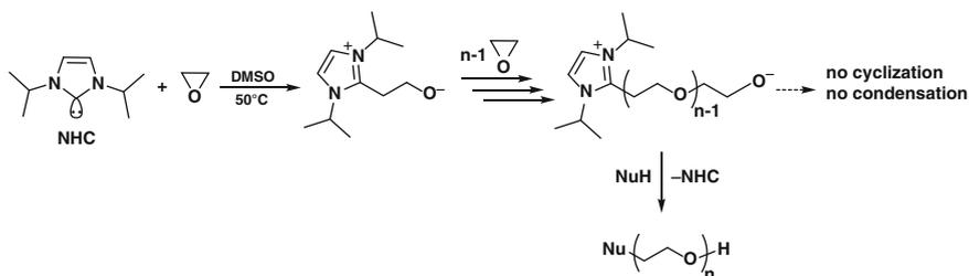
**Scheme 9** Proposed mechanism for ethylene oxide polymerization initiated by N-heterocyclic carbenes
