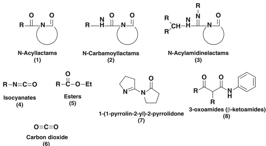
**Scheme 37** Main activators in anionic lactam ring-opening polymerization
