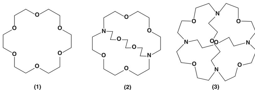
**Scheme 4** Crown ether 18C6 (1), cryptand 222 (2) and sphere (3) used to complex alkali metal cations in ethylene oxide polymerization
