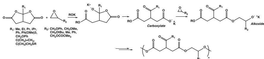
**Scheme 33** Bis( $\gamma$ -lactones) and epoxides for the synthesis of alternated copolymers
