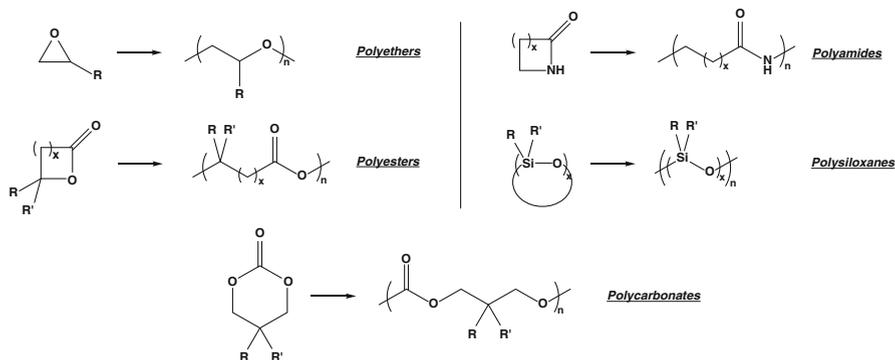
**Scheme 1** Ring-opening polymerization of main cyclic monomers
