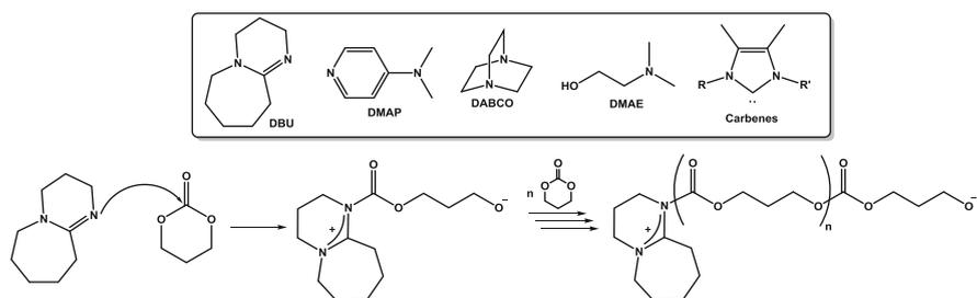
**Scheme 68** Examples of organic initiators for the AROP of 6-membered cyclic carbonates and polymerization mechanism
