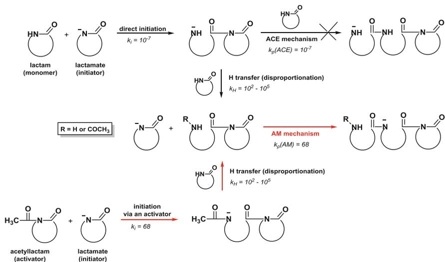
**Scheme 38** Formation of active species in anionic ring-opening polymerization of  $\epsilon$ -caprolactam: activated monomer (AM) mechanism vs. active chain-end (ACE) mechanism
