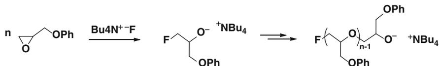
**Scheme 10** Polymerization of glycidyl phenyl ether initiated with tetrabutylammonium fluoride
