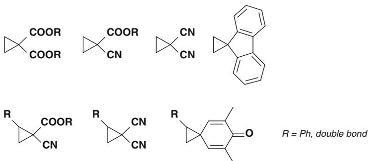
**Scheme 73** Structure of cyclopropanes polymerized by AROP
