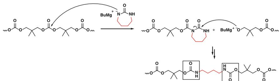
**Scheme 79** Polyurethane synthesis by insertion and ROP of deprotonated tetramethylene urea in a polycarbonate
