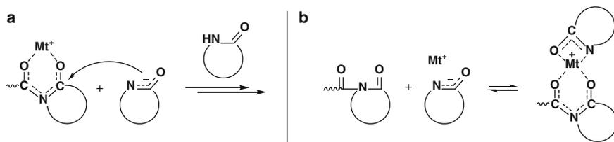
**Scheme 40** Lactamolytic (a) and ion-coordinative (b) mechanisms
