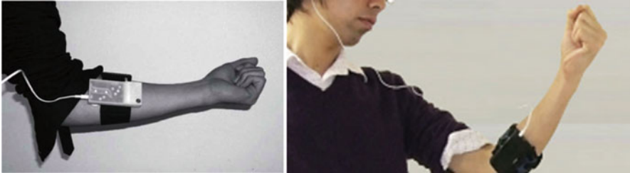
Fig. 7.7 BioTones: A wearable device for converting a person's bioelectrical signals on the basis of electromyogram signals into audio sounds. The device is capable of extracting the signals and generating audio sounds. The users can simply listen to the generated sound by using normal headphones
