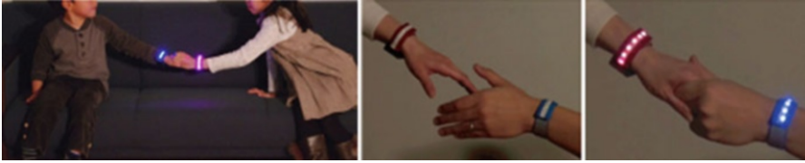
Fig. 7.9 Enhanced touch: This wearable device with electrodes senses touch and identifies other users. Six full-color LEDs are installed in the bracelet, which light up when a handshake occurs
