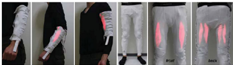
Fig. 7.5 BioLights: light emitting wear for visualizing upper and lower-limb muscle activity
