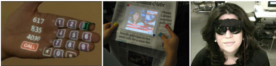
Fig. 7.4 SixthSense (left and center). A wearable gestural interface to combine the virtual and physical world. Expression Glasses (right). A wearable approach for facial expression recognition
