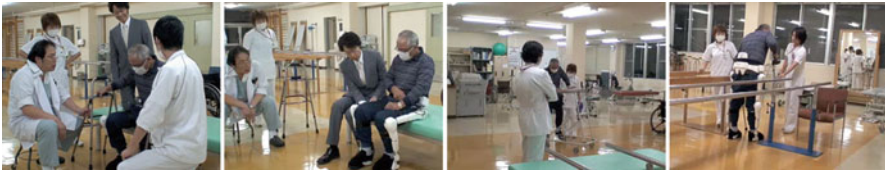
Fig. 1.4 HAL trials at the hospital. A patient succeeded in standing up, sitting down, and moving (bend and extend) his feet according to his intention by using HAL. He could also walk with walker and cane
