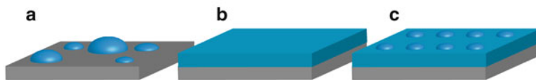
Fig. 17.2 Growth modes for thin film: (a) island growth or Volmer–Weber growth, (b) layer-by-layer growth or Frank van Merwe growth, and (c) Stranski–Krastanov growth
