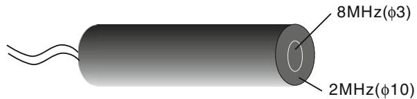
Fig. 7.2 Schematic diagram of a multi-wave TDX
