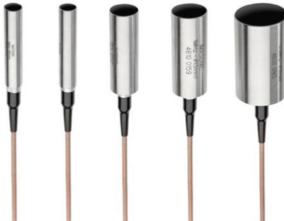
Fig. A.1 Photograph of ultrasonic transducers provided by Met-flow S.A. [8]
