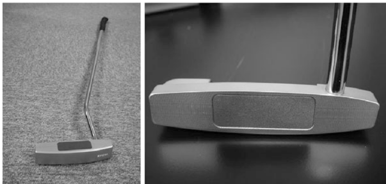
Fig. 10.23 Golf putter whose central part is made of lotus copper. This putter exhibits superior vibration–damping capacity. Players feel soft to hit a ball (Reprinted with permission from [16] © 2006 Elsevier Ltd)
