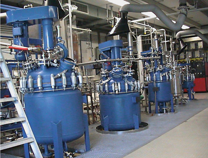
■ Fig. 4.1.11 Hyperthermophiles fermentation plant, University of Regensburg. Partial view, showing two 300 l and one 130 l fermenters
