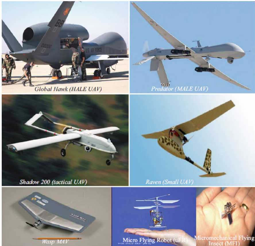
Fig. 1.17 Unmanned aerial vehicles, from big platforms to micro flying robots
