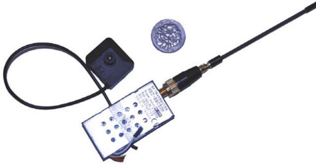
Fig. 3.5 Wireless camera system
