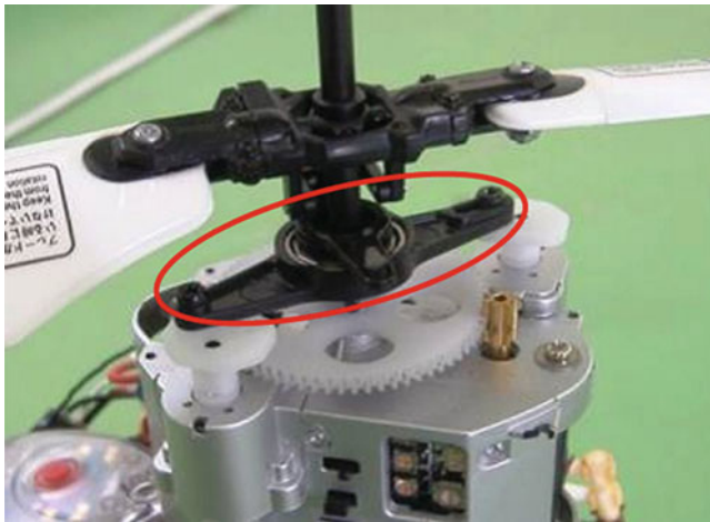
Fig. 2.4 Swash plate of coaxial-rotor helicopter
