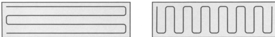
Fig. 3. The number of turns is the main factor in the cost difference of covering a region along different sweep directions.
