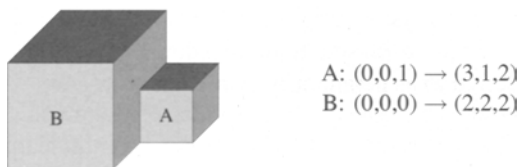
Fig. 2. This figure shows how a volume can be approximated with two overlapping bricks and how we represent this.
