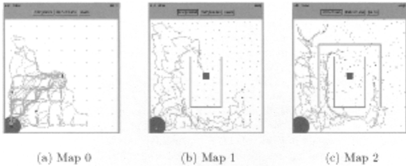
Fig. 1.3. The simulation environments. (a) Map 0 is the first obstacle-free environment. A sample configuration is shown with 81 embedded nodes distributed uniformly throughout the environment without any error in placement. (b) Map 1 is a more complicated environment with a box canyon. A sample configuration is shown with 225 embedded nodes distributed uniformly with .5 m of error in placement. (c) Map 2 the most complicated environment with two box canyons. A sample configuration is shown with 289 embedded nodes distributed uniformly with 10m of error in placement.
