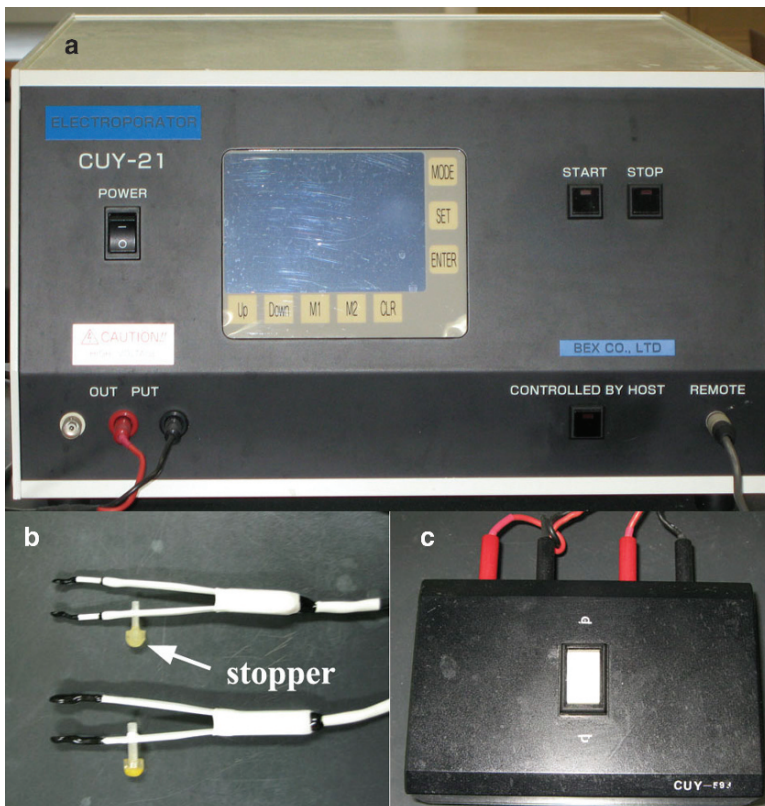
Fig. 24.3 Electroporator and forceps-type electrodes. (a) An electroporator. A pedal switch is helpful for energizing the testis. The diameter of the forceps-type electrodes must match the size of the target (b) . The stopper helps avoid rupturing the testis due to excessive pressure. A current direction selector is recommended for changing the direction of the current (c)
