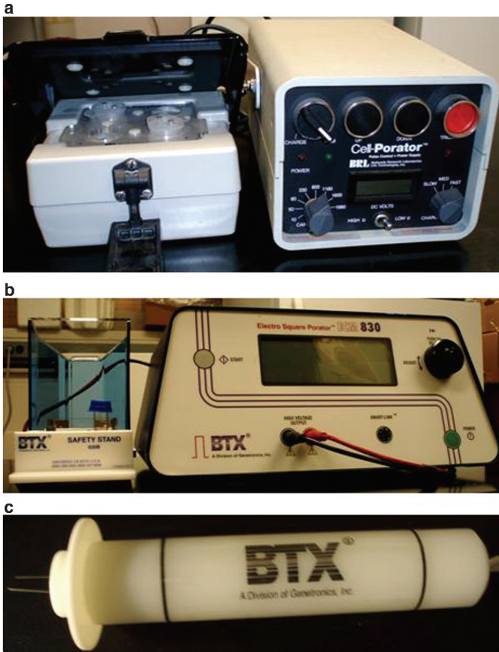
Fig. 20.1 Commercially available electroporators. (a) Exponential decay generator (Cell-Proator) from BRL, (b) a square wave generator from BTX, (c) hand-held electrode attach to the square wave generator from BTX
