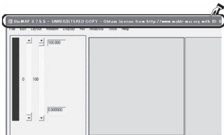
Fig. 9.1 BioMap is functionally locked before user registration. When “ID” is displayed in the upper part of the window, the functions of BioMap cannot be used. Activating the software at http://www.maldi-msi.org is necessary
