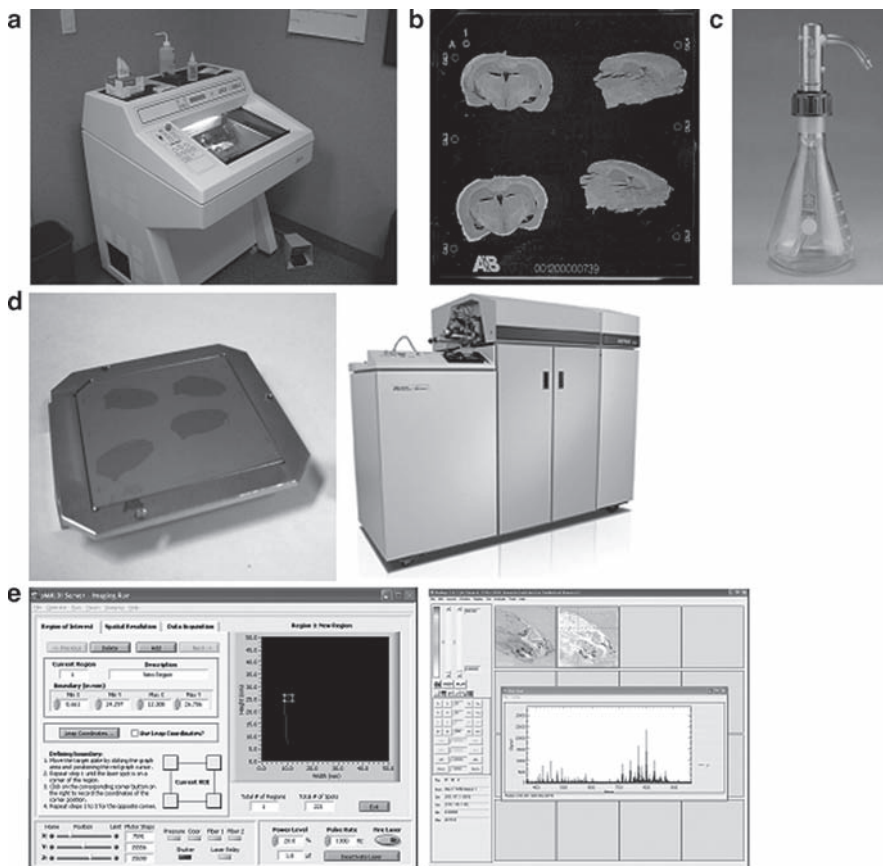
Fig. 14.5 Workflow for matrix-assisted laser desorption/ionization-mass spectrometry (MALDI-MS) using the QSTAR Elite system: slice tissue sections ( a ), mount sample to plate ( b ), spray-coat with matrix ( c ), load sample plate into QSTAR Elite system ( d ), and perform data acquisition using oMALDI server 5.0 software and processing with BioMAP software ( e )
