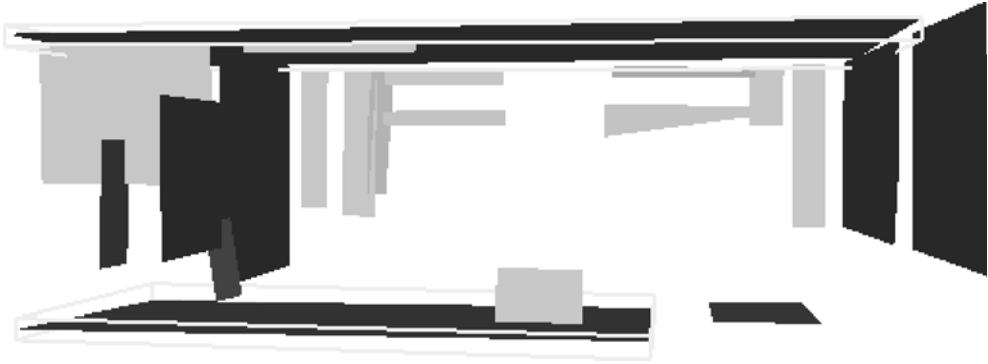
Figure 5.10 Planes extracted from the 3D point cloud of figure 5.9. The ground and ceiling plane are marked by a bounding box.
