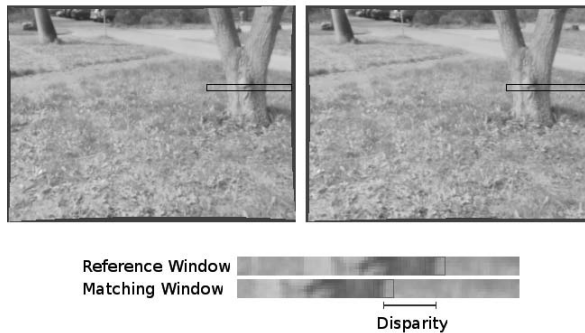
Figure 3.37 Window-based stereo vision
