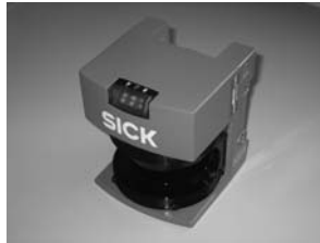
Figure 3.30 The Sick laser scanner LMS200
