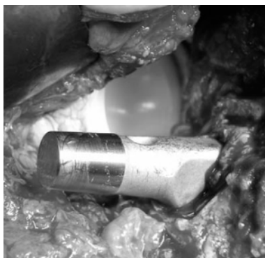
Figure 2: Example for a grade 2 damaged taper.
