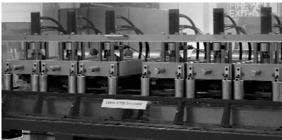
Figure 1: Leeds II Physiological Anatomical hip joint simulator.
