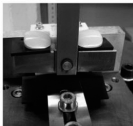
Figure 9: Static strength test for 'Wedge Load'.
