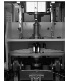
Figure 2: Pendulum friction simulator.
