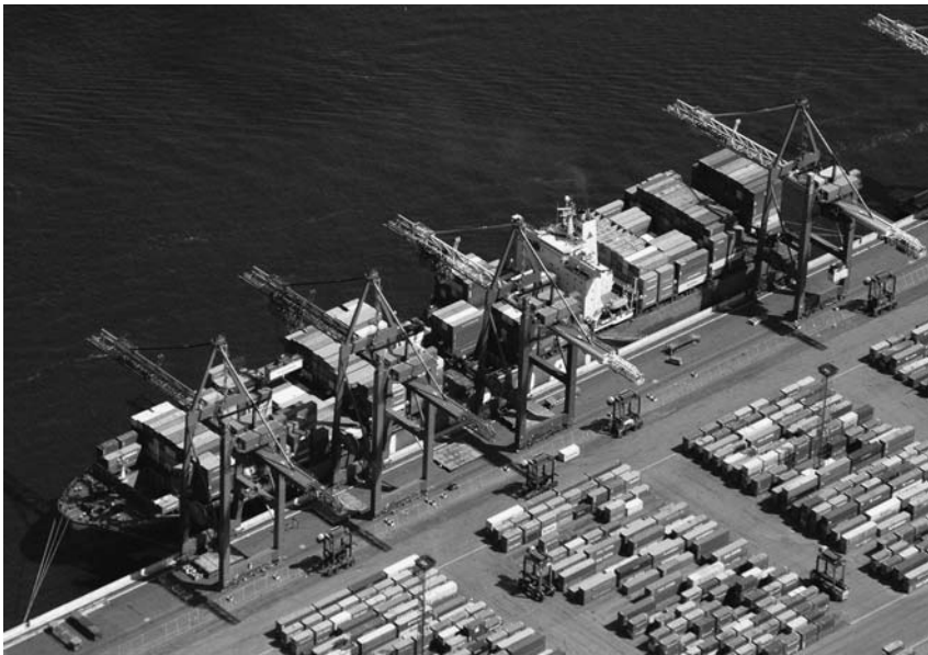
Fig. 2.6 Quay cranes serving a container vessel (source: Port of Hamburg Marketing / D. Hasenpusch, 2008)
