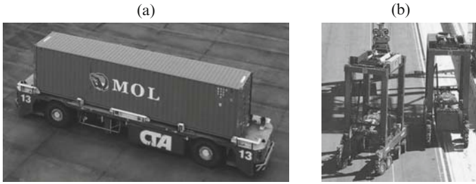
Fig. 2.8 AGV at the port of Hamburg (a) and ALVs at the port of Brisbane (b) (source: Gottwald Port Technology, 2008; Kalmar Industries, 2008)
