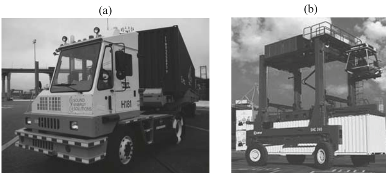
Fig. 2.7 Yard truck (a) and straddle carrier (b) (source: Kalmar Industries, 2008)
